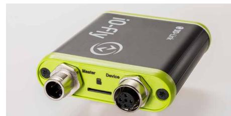
The device provides connection options for an IO-Link device and in IO-Link master as well as a slot for a Micro SD card.
