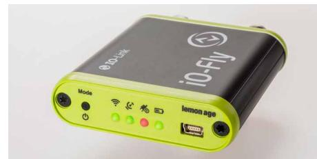
Colored LEDs provide information about the status of the iO-Fly, the battery charging status, the connection to the IO-Link device as well as the type of established wireless connection. The integrated battery can be charged via a USB port.
